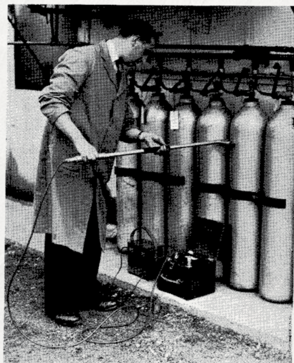
Fig. 8. Portable Level Detector employing a Gamma Rag Source and Geiger-Müller Tube.
