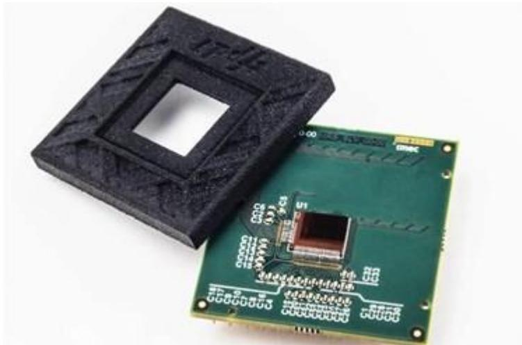
Until recently short-wave infrared (SWIR) image sensors have been produced using a hybrid technology in which a III-V-based photodetector, usually InGaAs-based, is flip-flop bonded to a silicon readout circuit. The resulting sensor is often highly sensitive, but the technology is expensive for mass manufacturing and limited in both pixel size and number of pixels,
